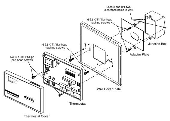
Figure 8. Mounting 1F60 thermostat to vertical junction box
